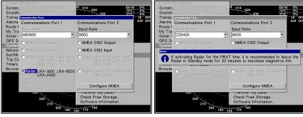
Communications Port menu (left). Radar Notice (right) prompting users to leave radar in Standby Mode for 30 minutes when activating radar for the first time.
